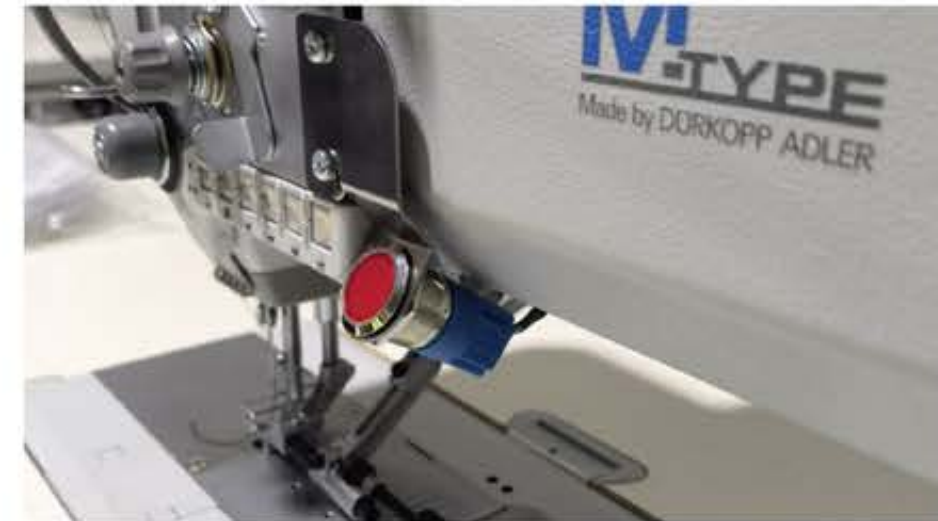
•Product design of emergency stop switch for sewing machine
